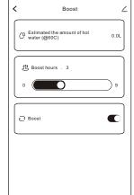
Select number of boost hours. Unit enters Standby mode after selected time/ tank is heated.
