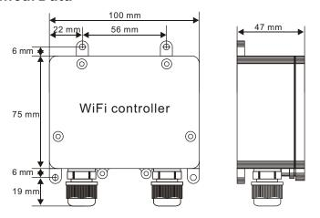
WiFi Controller is waterproof and UV rated for outdoor installation.
