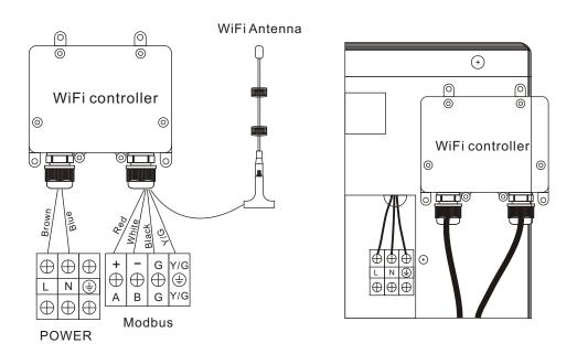
Note: Controller must be mounted vertically with cable access facing down. Ideal location is at rear top on right hand side of the heatpump (fixing tape) however 2m cables make remote mount also possible (screws provided). Wi-Fi antenna must be installed outside of heat pump. It has a magnetic base so can be mounted on the lid of the heat pump or any surface without frequency interference.
