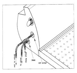
The tubing from the heat exchanger to the solar system is connected as shown in the diagram. A kit containing the fittings required to make these connections is available from your SOLCO SOLARTECH Genius consultant.
