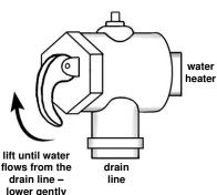
If water does not flow freely from the drain line when the lever is lifted, then the water heater must be checked. Phone Rheem Service or their nearest Accredited Service Agent to arrange for an inspection.
