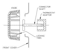
Align the knob slots over the 'T' drive on the connector shaft, with the dial at the lowest setting – a firm push with the hand on the knob front face will engage the locking tabs.
