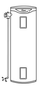
⚠ Warning: Never replace the relief valve with one of a higher pressure rating.
