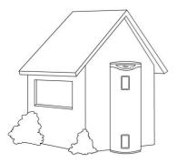
It is recommended the water heater be installed at ground or floor level and must stand vertically upright. The base of the water heater is made of corrosion resistant material, and it may be placed directly in contact with the supporting surface. It is not necessary to allow for free air circulation under the base of the water heater.
