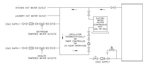
NOTE: A PLV IS REQUIRED TO BE INSTALLED ON THE COLD SUPPLY LINE TO THE TEMPERING VALVE IF A PLV IS INSTALLED ON THE COLD SUPPLY LINE TO THE WATER HEATER.
