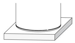
A properly drained overflow tray must be used where property damage could occur from water spillage. (See AS/ NZS3500.4 for further details.)
