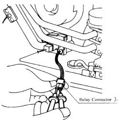
a.) Disconnect relay connectors  $(J_4)$  and  $(J_5)$  and measure resistance between White and WhiteW on heater side (water flow servo and HW connection).
