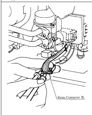
a.) Disconnect relay connector (B<sub>1</sub>) and measure resistance.
