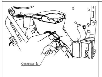
a.) Measure voltage between Grey and Black of connector  $(J_6)$ .
