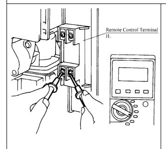
Check the voltage between the 2-core remote control cable.
