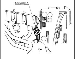
b.) Measure the voltage of the connector (A) on the PCB.
