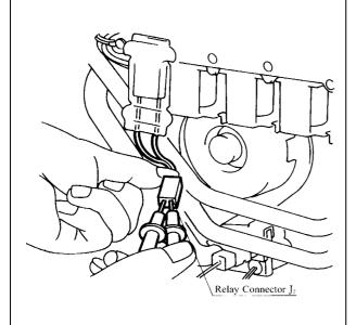
a.) Disconnect relay connector  $(J_2)$  and measure resistance between Blue and Blue.
