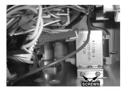
d. Remove transformer installation bracket screw.
