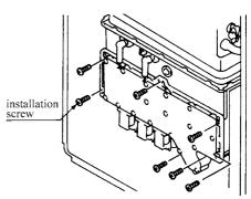
4) Replace the manifold (complete assembly) and the packing. (7 screws)
