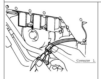
a.) Disconnect Solenoid Valve 2 connector and measure resistance between Orange and Black.
