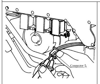
a.) Disconnect Solenoid connector, measure resistance between Yellow and Black.
