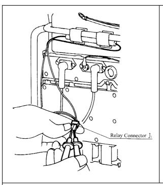
c.) Disconnect relay connector (J1) and (J3) and measure resistance between Yellow and Yellow on Heat Exchanger Heater side.
