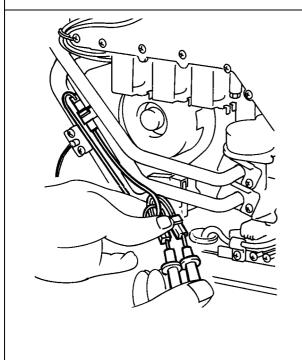
b.) Disconnect relay connector  $(J_4)$  and  $(J_5)$  and measure resistance between Yellow and Yellow on each conector on heater side.
