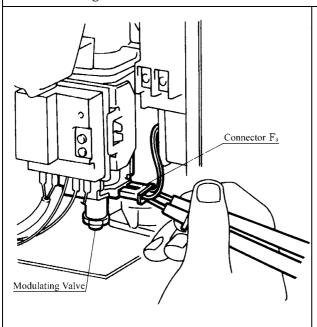
a.) Disconnect Modulating Valve fasten terminal and measure resistance between terminals.
