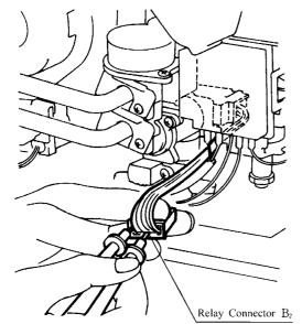
a.) Disconnect relay connector (B<sub>2</sub>), and measure resistance between Red and Blue of Water Flow Servo.
