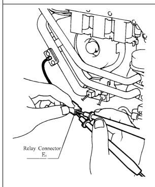
Check Hot Water Thermistor if error code 32 is displayed.
