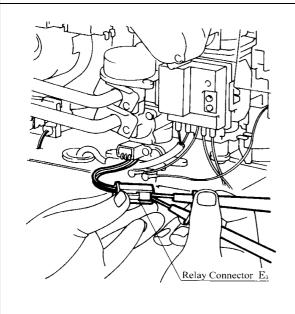
a.) Measure voltage between Red - Black of relay connector  $(E_3)$ .
