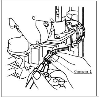
Check the main solenoid if error indicator "11" is displayed.
