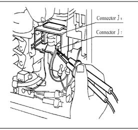
a.) Measure voltage between blue and brown on the connecter J<sub>7</sub>
