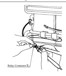
Check Heat Exchanger Outlet Thermistor if error indicator "33" is displayed.
