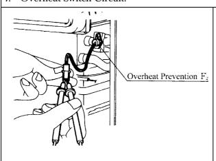
Measure resistance between Overheat Switch terminals (F<sub>2</sub>).
