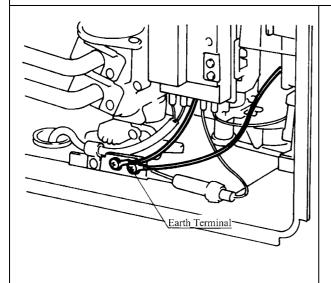
Confirm the Earth Lead connection is secure (at round terminal), and check for broken or short circuits in the lead.
