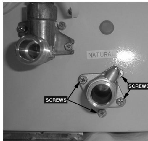
d. Remove one (1) gas control (assy) screw and pull out gas control (assy).
