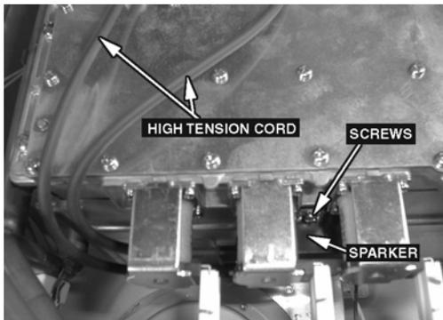
5) Removal of the **Combustion Fan**
