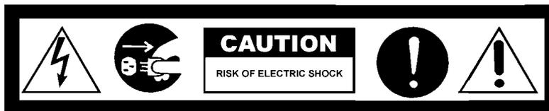
*240 volt potential exposure. Isolate the appliance and reconfirm with a neon screwdriver or multimeter.*
