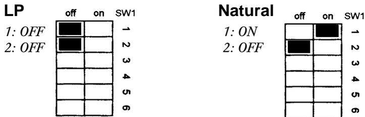
Note : Only alter gas type positions when converting from one gas type to another. For gas conversion instructions refer to page 41.
