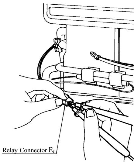
Check Heat Exchanger Outlet Thermistor if error indicator “33” is displayed.
