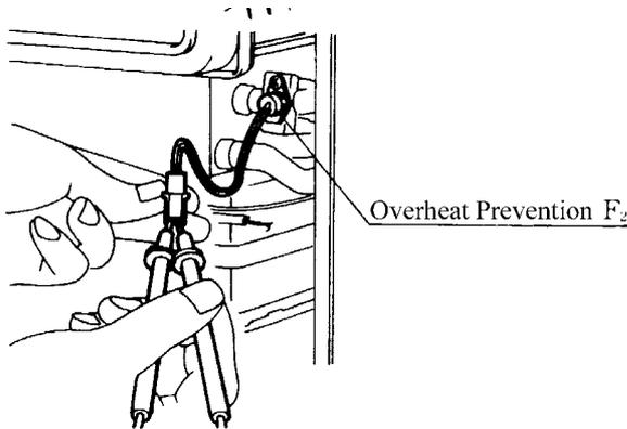
Measure resistance between Overheat Switch terminals (F<sub>2</sub>).
