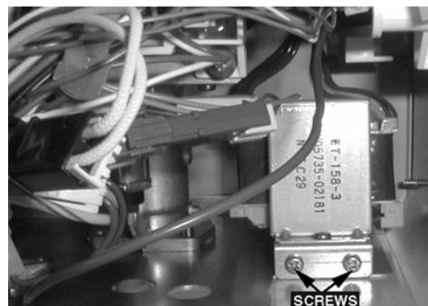
d. Remove transformer installation bracket screw.
