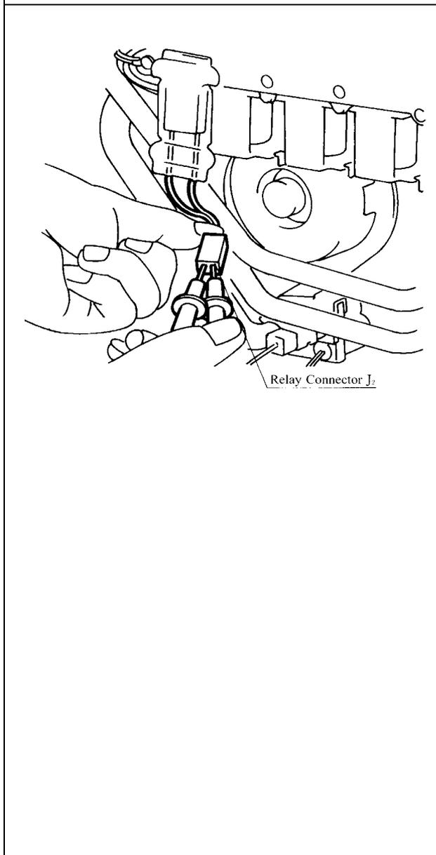
a.) Disconnect relay connector (J2) and measure resistance between Blue and Blue.
