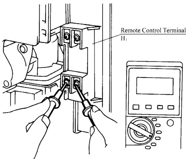
Check the voltage between the 2-core remote control cable.
