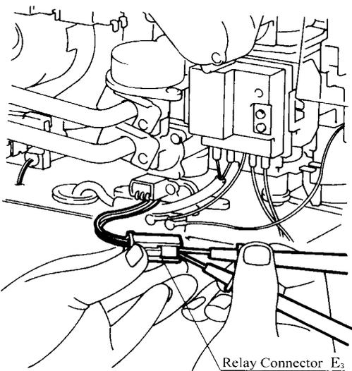
a.) Measure voltage between Red - Black of relay connector (E<sub>3</sub>).
