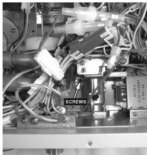
**10) Removal of the Heat Exchanger**
