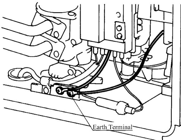
Confirm the Earth Lead connection is secure (at round terminal), and check for broken or short circuits in the lead.
