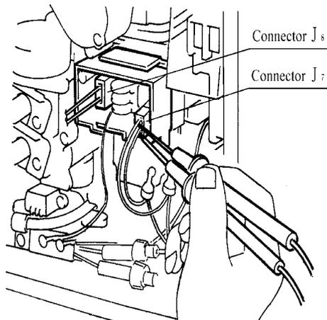
a.) Measure voltage between blue and brown on the connector J<sub>7</sub>
