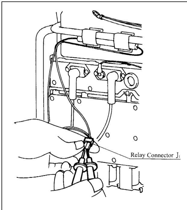
c.) Disconnect relay connector (J1) and (J3) and measure resistance between Yellow and Yellow on Heat Exchanger Heater side.
