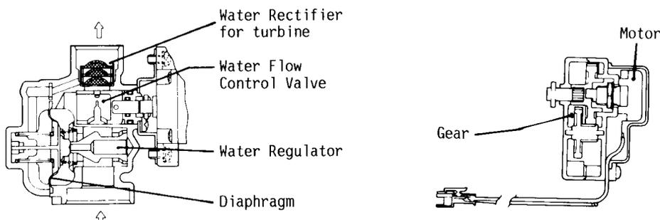
The water flow through the heat exchanger is dependant on the incoming and outgoing water temperatures, the P.C.B. controls the settings of the water flow control valve to provide the correct flow for the conditions at any given time.
