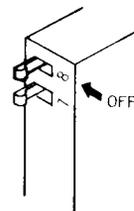
**NOTE:** Switches 5, 6, 7, & 8 should be in the OFF position, upon completion of setting the pressure. Only the correct gas selection switch for the area of installation should remain in the ON position.
