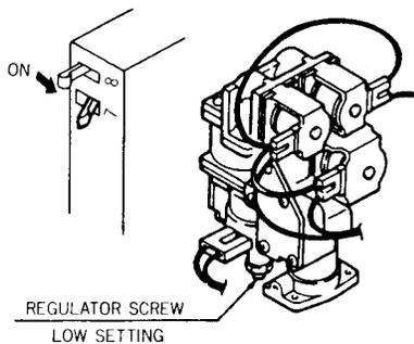
6. After having adjusted the potentiometer to achieve the correct pressure setting, return the No.8 switch to the OFF position.
