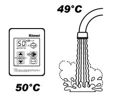
Depending on the weather conditions and the length of the pipe between the hot water unit and the outlet in use, there may be a variation between the temperatures displayed at the water controller(s) and the temperature of the water at the outlet.
