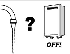
At low water flows, the hot water unit may extinguish without warning. Opening the tap further will restart the appliance.
