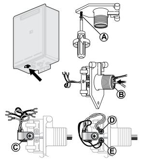
'Ezi connect' cable connector for water heater models: INFINITY 32, 26i, ENVIRO & HD/HDC Series
