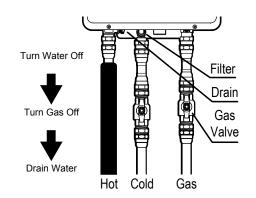
If freezing conditions are expected, turn off water and gas and drain all water from the appliance. If power and the automatic frost protection are connected, freezing will be prevented. (Anti-frost protection is fitted as standard equipment on External units and is available as an optional extra on Internal Units).
