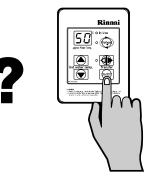
There is no need to turn the water controller(s) off after use. However, if you prefer to turn the water controller(s) off, selected temperatures to a maximum of 50°C will be stored in the system memory at all times whilst mains power remains connected.
