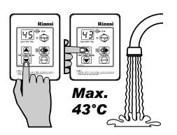
Whilst hot water outlets are open the set temperature may be lowered. However they cannot then be raised above 43°C. In addition transfer of 'priority' between controllers is not possible. These are safety features.
