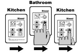
As a safety precaution, if a Kitchen Controller's temperature is set above 50°C, transferring and then returning 'priority' to the Kitchen Controller will result in a default set temperature of 50°C being selected. This is a safety feature.
