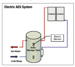
water temperature falls below 60°C and will only consume electricity until the water temperature is increased to 60°C then turns off again.
