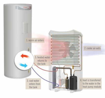
When power is available, the Heat Pump heating cycle will continue until the tank is full of hot water.
