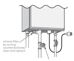
turn off the water inlet supply valve then turn on a hot tap to release the pressure
